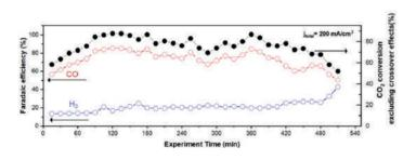
Denmark Techinal University was able to show ~80% conversion of CO<sub>2</sub> to CO for 8 hours (excluding CO<sub>2</sub> crossing over to the anode)
