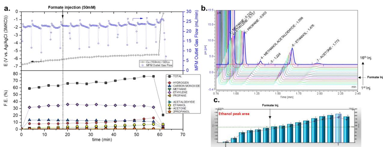
Figure 5: a) Cathode potential, outlet gas flow and faradaic efficiency of the products over the course of 1h experiment with **formate** injection between the 4<sup>th</sup> and 5<sup>th</sup> injection, b) waterfall plot of GC injections with an emphasis on the C<sub>2</sub>+ liquid products, c) Bar-graph of Ethanol peak area at each injection
