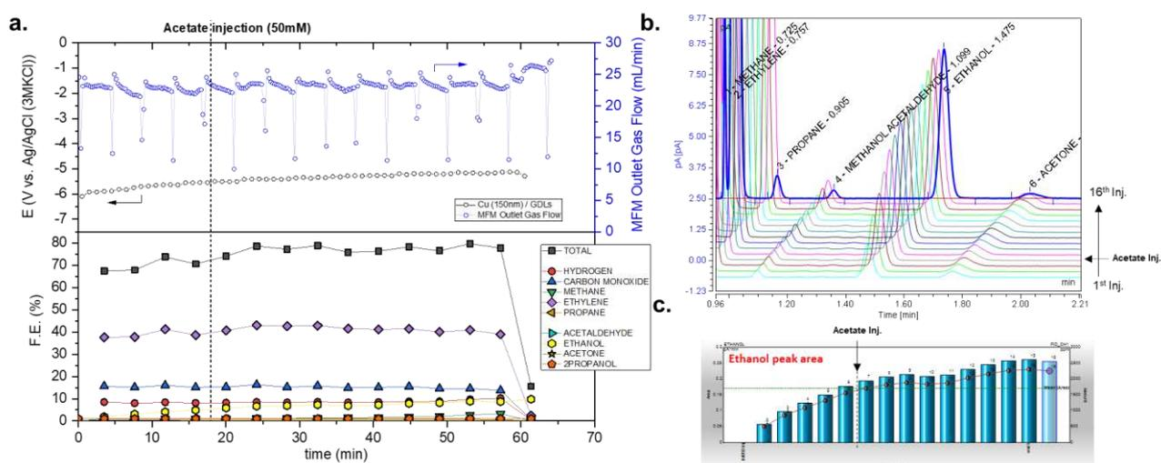
Figure 6: **a)** Cathode potential, outlet gas flow and faradaic efficiency of the products over the course of 1h experiment with **acetate** injection between the 4<sup>th</sup> and 5<sup>th</sup> injection, **b)** waterfall plot of GC injections with an emphasis on the C2+ liquid products, **c)** Bar-graph of Ethanol peak area at each injection
